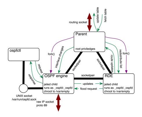
The OSPF Engine communicates with the neighbors and runs all the finite state machines. The periodic hello messages are generated by the OE. Updates are passed to the Route Decision Engine. The RDE calculates the SPF (shortest path first) tree and based on this info the RIB is generated. Updates are passed to the parent process for the FIB and to the OE so that the updates are flooded on through the network.
