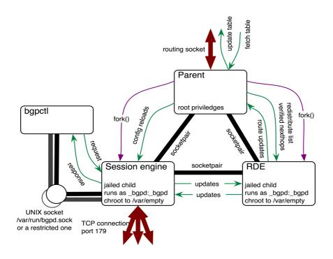
The Session Engine communicates with all neighbors and sends out the keepalive messages. Updates are passed to the Route Decision Engine where the filtering and routing table calculations are done. Changes in the RIB -- the Routing Information Base -- are sent to the parent process to update the FIB -the Forward Information Base -- and to the SE to send updates out to the neighbors.
